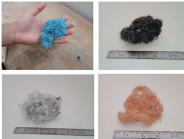
Figure 19: Fleece obtained with recycled polypropylene pellets (blue) and recycled PLA fleeces in black, white, and orange.
