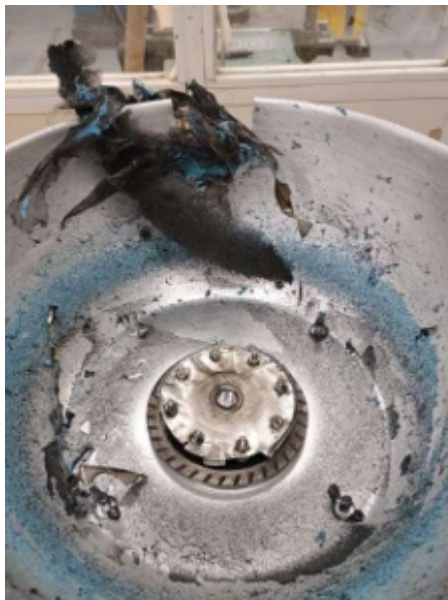
Figure 9: An accident occurred with the use of a can. Only the bottom of the can remained fixed to the cutting disc.
