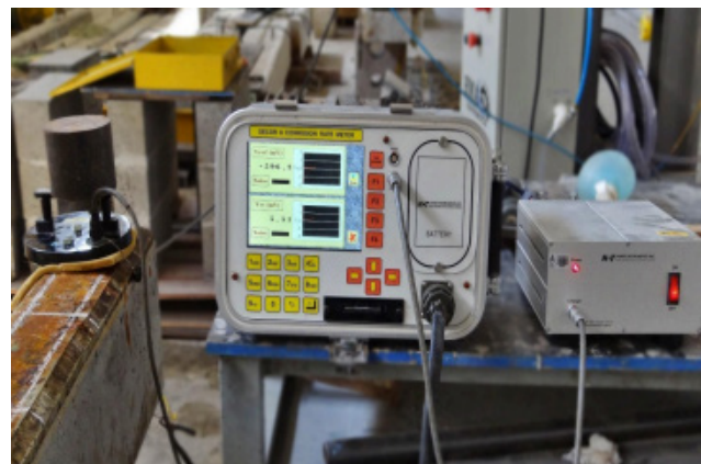
Figure 5: Determining the corrosion potential with the GECOR 8 equipment.
