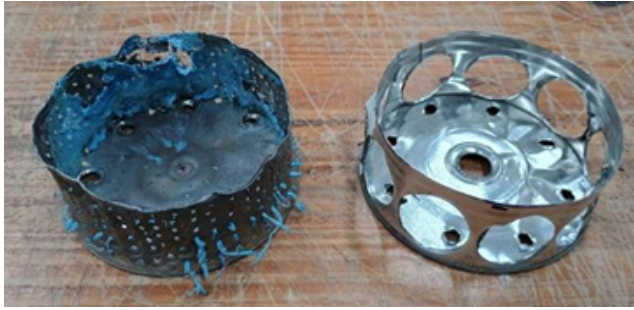
Figure 8: Emitter cup used in the first tests. Researchers manufactured the first two attempts using powdered milk cans, first making small holes in the can itself with a drill (left) and then making larger holes and using a cornmeal sieve as a screen to disperse the threads.
