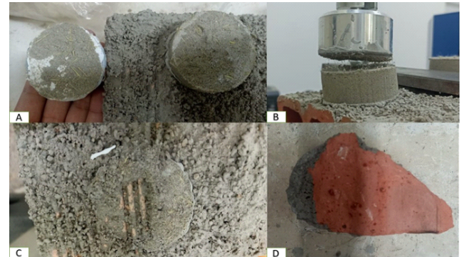
Figure 10: Visual appearance of fractured specimens.
