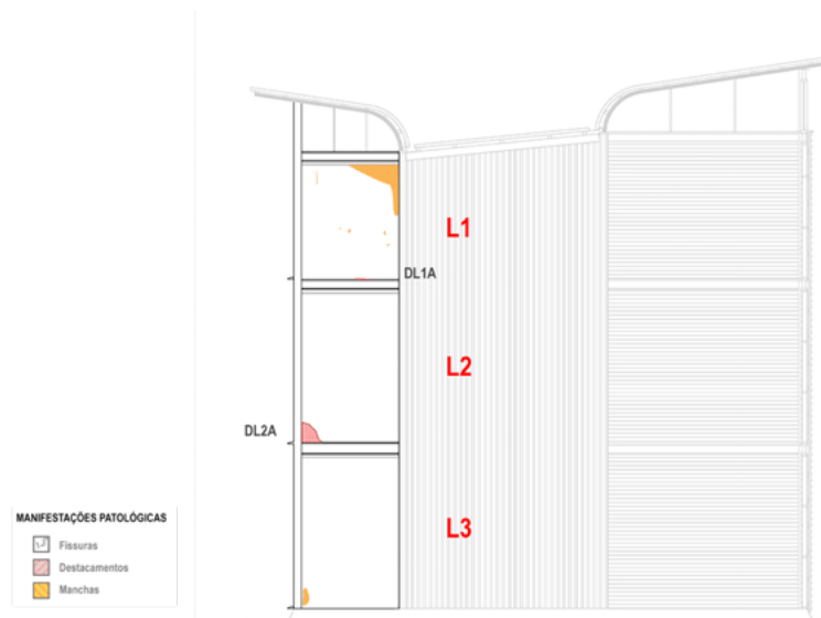
Figure 14: Pathological Manifestations on the East Façade (Unit 001). Source: Elaborated by the Authors (2022)
