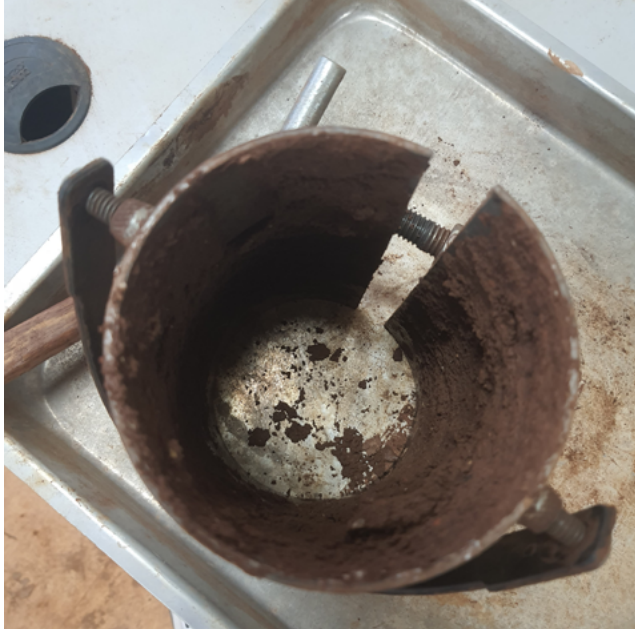
Figure 2: Adherence of the mixture (0% - Group 1) to the mold. Source: Authors.
