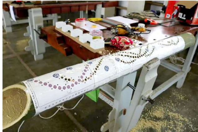
Figure 4: Mold attached to bamboo thatch. Source: Personal collection of Silvia Sasaoka (2020).
