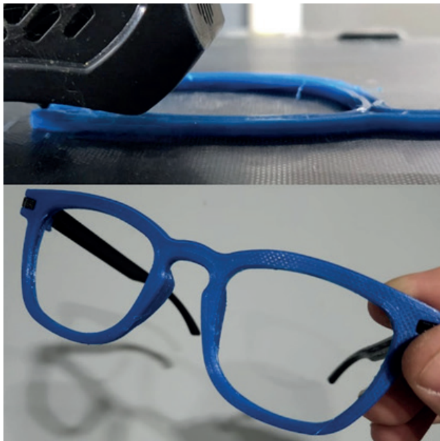
Figure 08: Printing with recycled PLA filament and Glasses printed with filament made from recycled PLA. Source: Authors.
