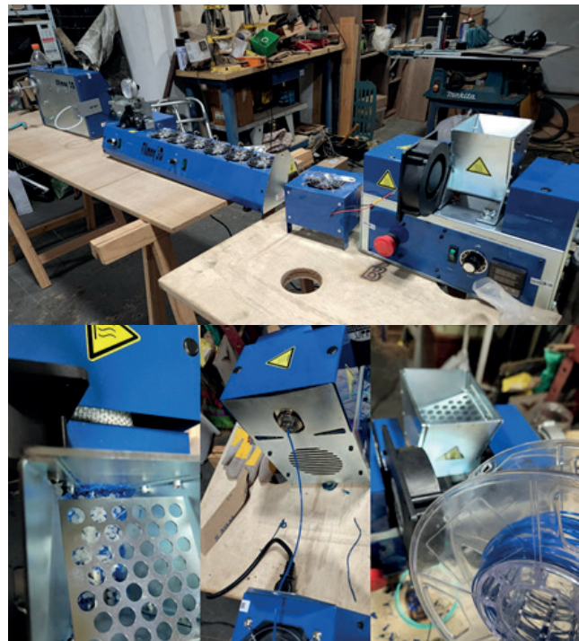
Figure 07 : Filament manufacturing process. Above: Filament manufacturing system. Below: From left to right: Introduction of virgin pellets and flakes; extrusion; filament ready for use. Source: Authors.
