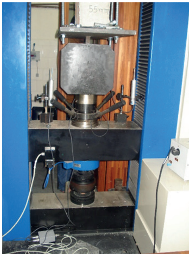
Figure 04: Universal testing machine, capacity of 300 kN. Source: Authors' collection.
