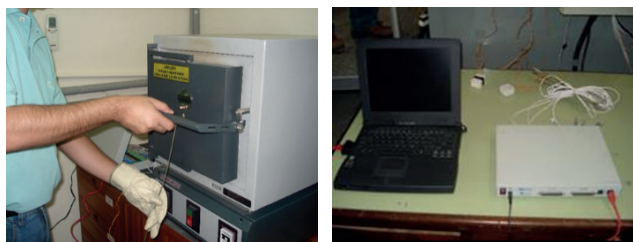
Figure 03: Thermocouples in the muffle furnace and the Data Acquisition System. Source: Authors' collection.
