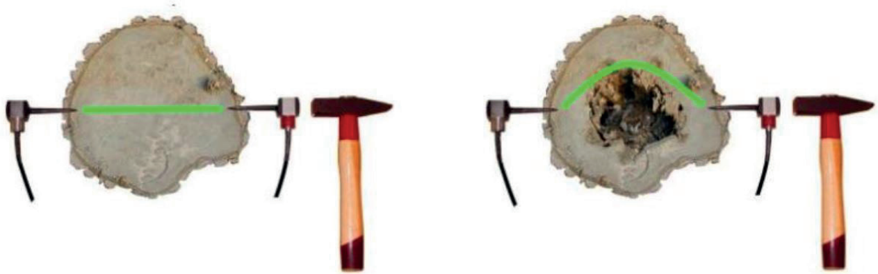
Figure 1: Path followed by the sound wave inside the wood. Source: Fakopp (2020).
