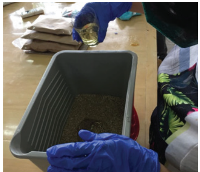
Figure 3: Manual blending of castor bean resin with the granules of the ground acai stone. Source: Authors (2018).
