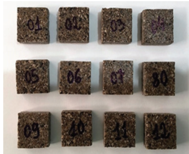
Figure 6: Test specimens for the density test, 25 mm x 25 mm. Source: Authors (2018).
