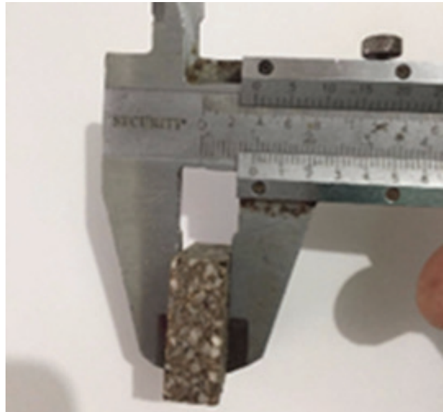
Figure 7: Measurement of thickness at the center of the sample. Source: Authors (2018).
