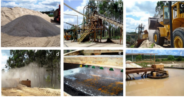
Figure 12 - Treatment of BA for recycling in mortars. MC1: material cycle 1 (conventional sand); MC2: material cycle 2 (BA generation); MC3: material cycle 3 (BA treatment and shipping to recycling); (a) BA storage; (b) conveyor belt material and power control unit; (c) BA introduction in washing system; (d) dust/particulate matter emission from BA; (e) water sprinkler system (showers); and (f) settling system for solids after BA washing
