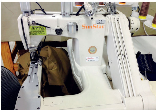
Figure 01 – Development of the first seam – Double Chain Stitch Sewing Machine Fonte: Author.
