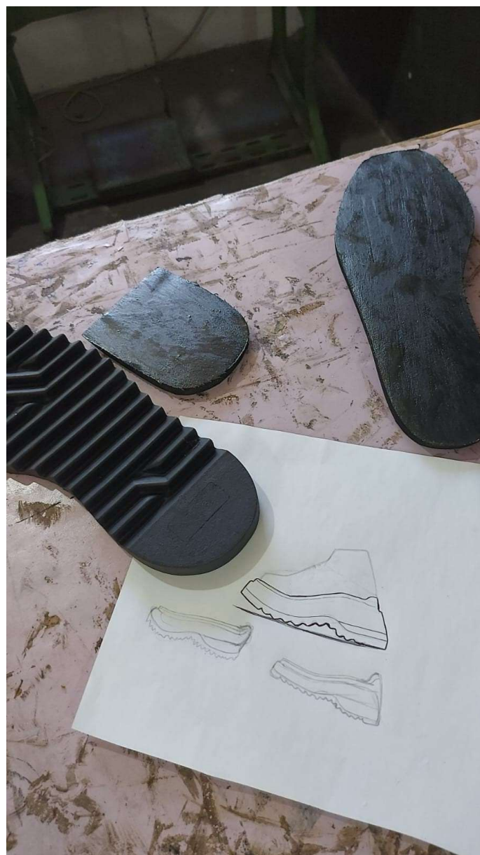
Figure 5 – Sole Design Process and Prototype for the Derby Shoe Model Redesign
