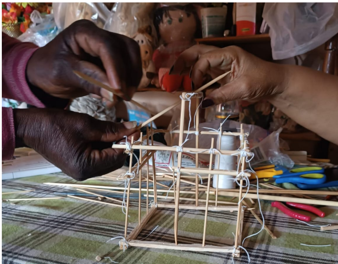
Figura 5 – Schematic 3D model of the construction of a wattle-and-daub structure of a traditional building in Salinas
