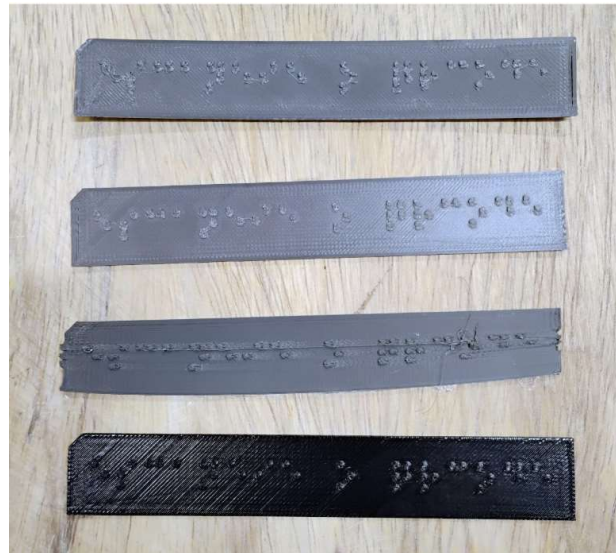
Figura 10 – Braille plate printing tests, in order of production.
