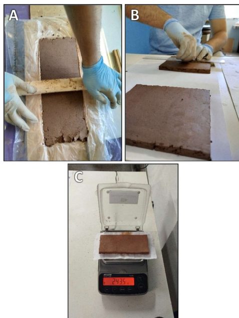
Figure 6 – Test specimen manufacturing: (A) shaping the mixture in the template; (B) cutting the mixture into a 5x15 sample; (C) weighing the wet sample.
