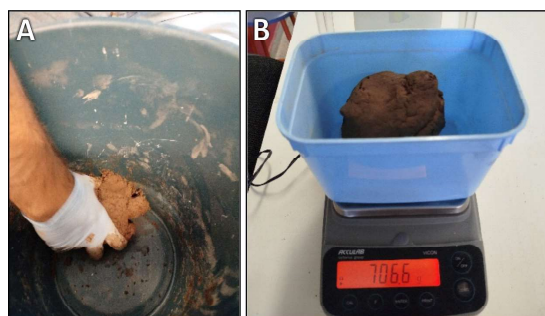
Figure 5 – Mixing for test specimens: (A) homogenization and (B) weighing.
