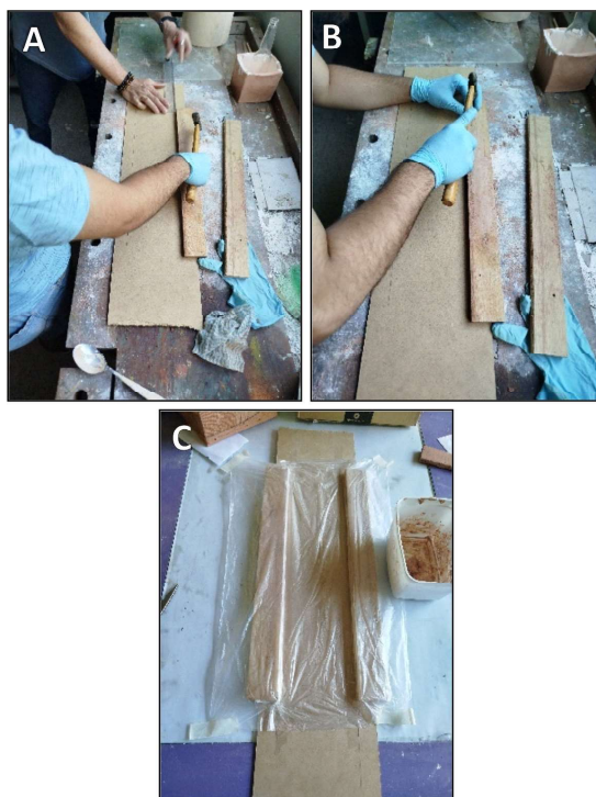
Figure 3 – Clay template construction process: (A) Aligning the guides; (B) Fixing the glides; (C) Ready template with plastic insulation.
