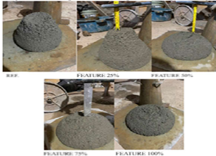
Figure 1 – Slump tests of all replacement percentages
