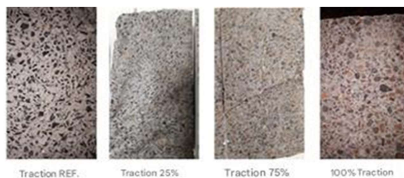
Figure 13 – Specimens after the splitting tensile strength test
