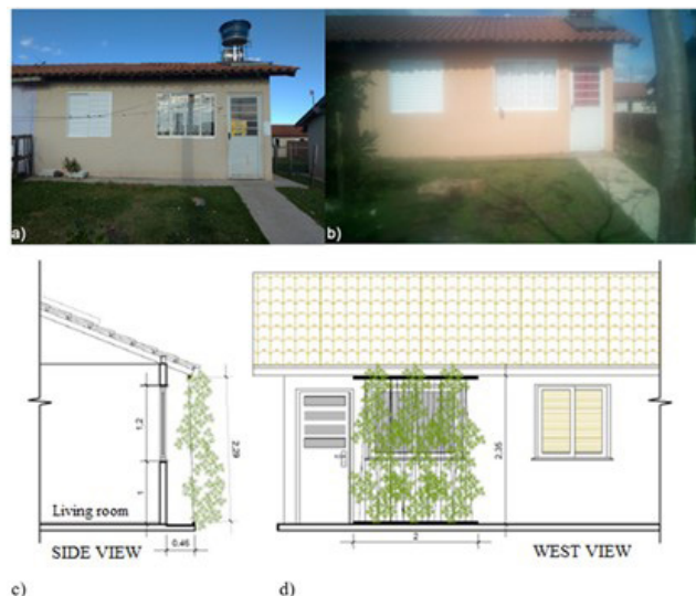
Figure 2: Position of green façade. a) and b) House units. c) side view of plant layer. d) west view of plant layer.
