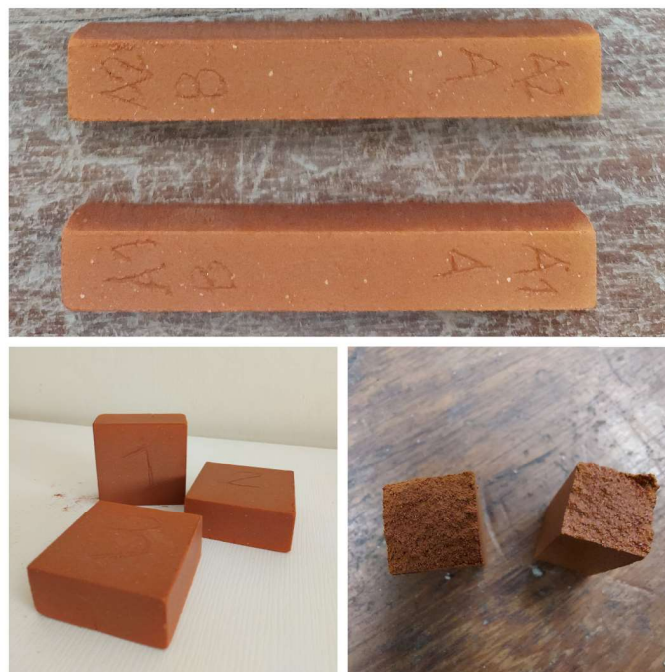
Figure 7 – Porous ceramic predominantly from Dredged Mud
