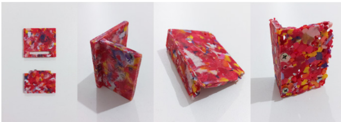
Figure 5: Fitting, welding, and screwing.
