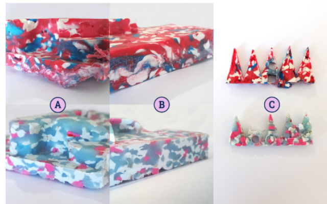
Figure 4: Sanding (A), saw cutting (B), and laser cutting (C) tests.
