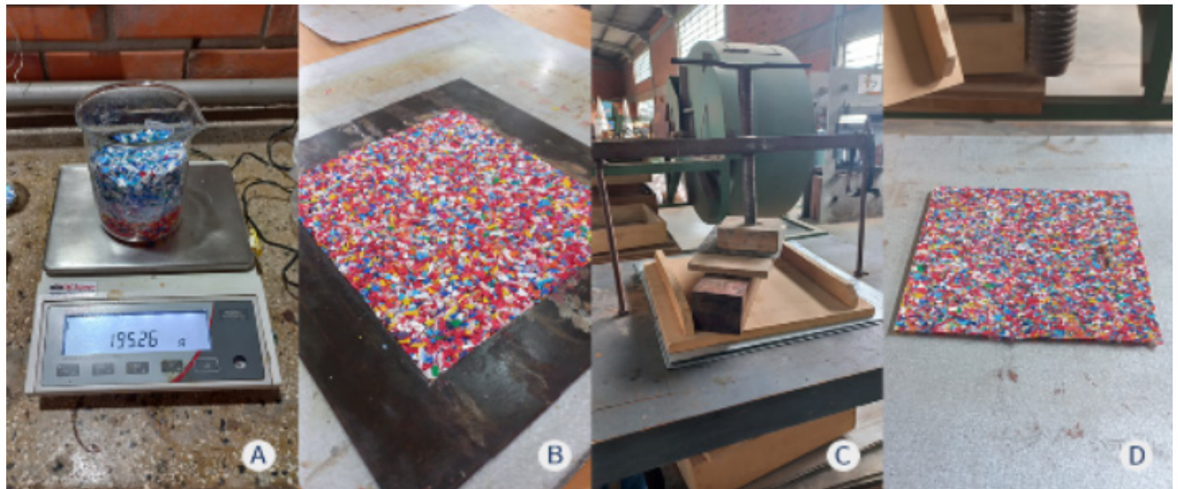
Figure 8: Weighing the material (A), placing it in the mold (B), placing it in the cold press after being removed from the hydraulic press (C), finished panel after being unmolded (D). Source: The Authors.
