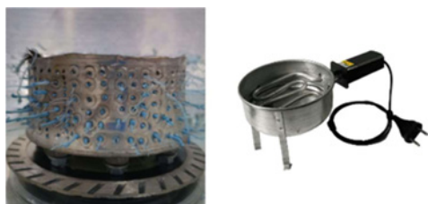
Figure 10: Detail - the space between the bottom of the cup, the base disc (left), and the stove used to help melt the plastic (right).
