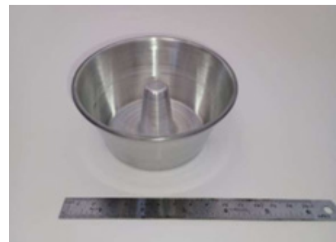
Figure 15: Mini pudding mold used to channel air. A hole was made in the central part for air passage.
