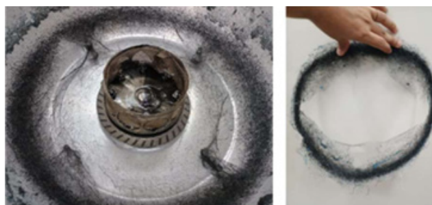
Figure 11: The high temperature melted the plastic, leaving it very fluid, leaving a solid residue on the container wall.
