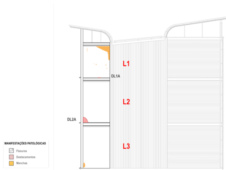
Figure 14: Pathological Manifestations on the East Façade (Unit 001).
