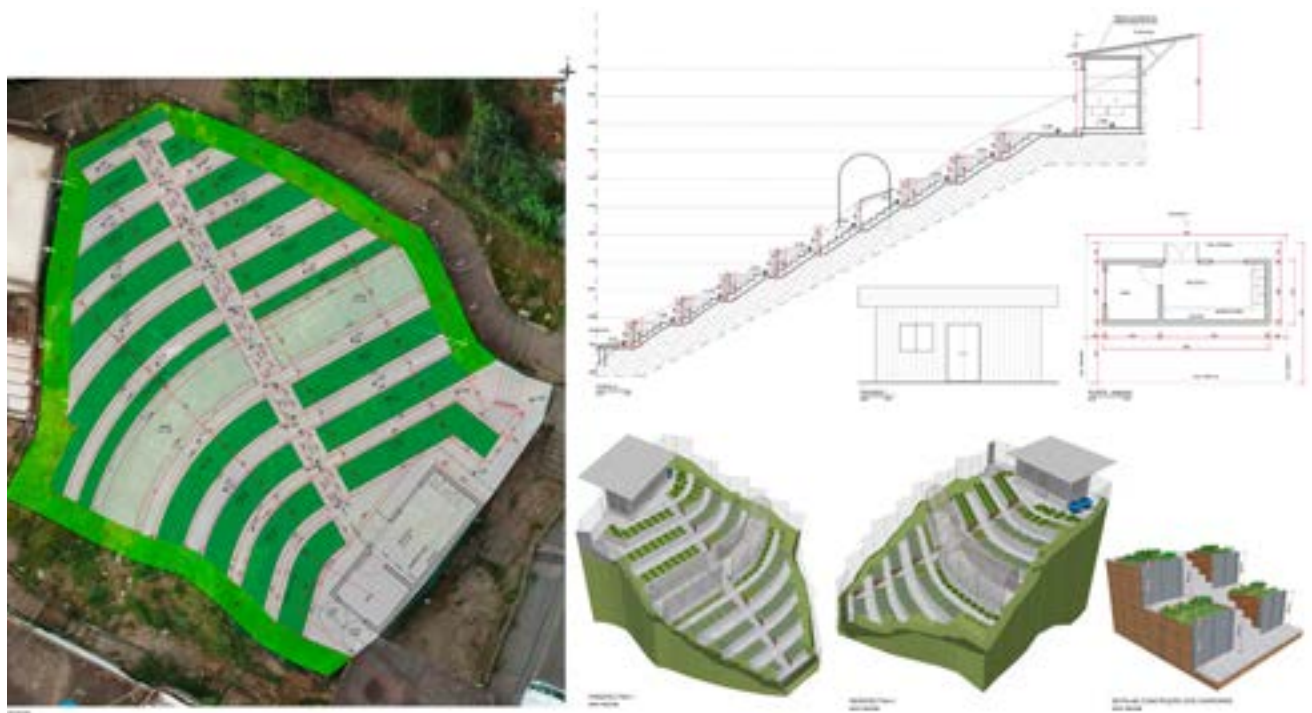
Figure 2: Planning for intervention in the Top Garden - a) plan (left); b) section along the terrain (top right); c) façade and plan of the social area (middle right); d) perspective views of the Garden and detail of the stairs and flowerbeds (bottom right). Author: Rosângela Mendonça/ ArquiCAD.
