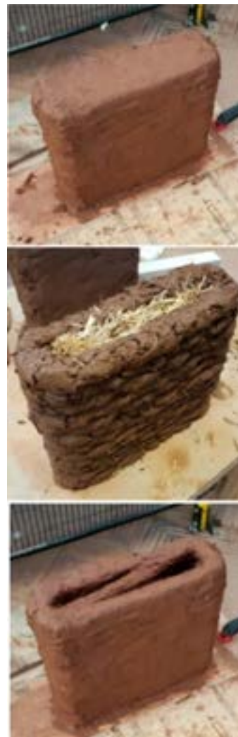
Figure 8: Solid prototype, single slit prototype with straw filling and double slit prototype. Source: (GOMAA et al. , 2019)
