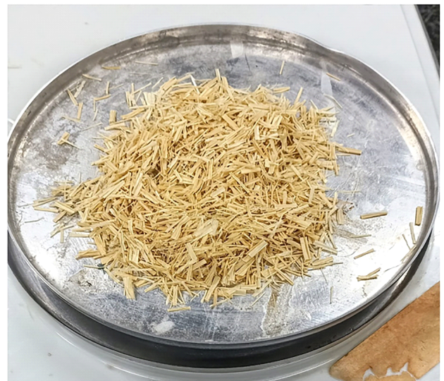
Figure 1: Tucumã fibers: (a) Commercially available product, and (b) After preparation for testing Source: Authors.
