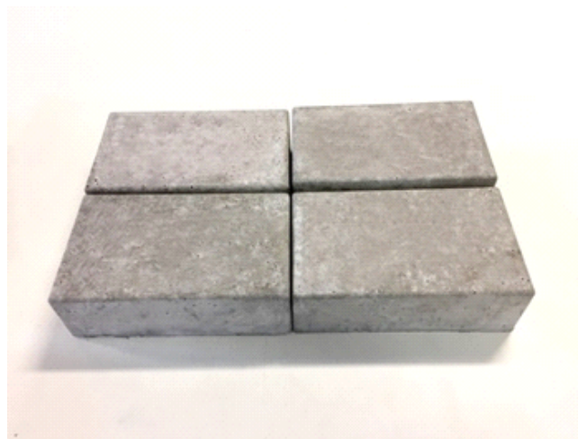
Figure 1: Shows some of the rectangular concrete blocks produced by SFS trace, with dimensions of 8 x 15 x 25 cm.
