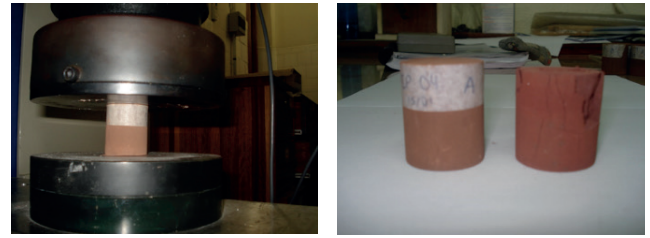
Figure 05: Detail of TS during the test and TS after the test.
