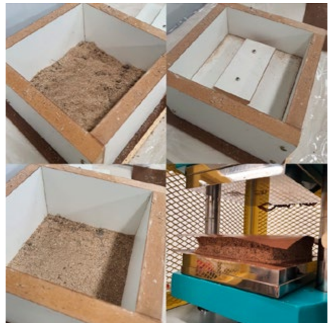
Figure 08: Shaped Fibers Ready for the Press. Source: Authors.
