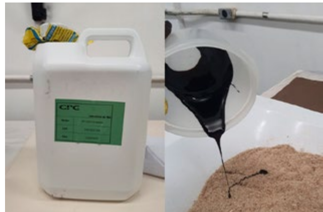
Figure 05: Lignin-Based Resin. Source: Authors.
