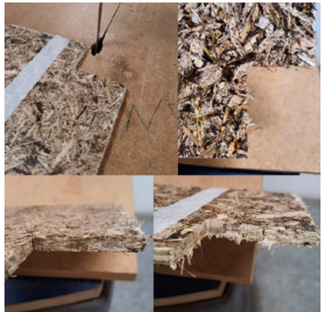
Figure 12: Machining with Band Saw.
