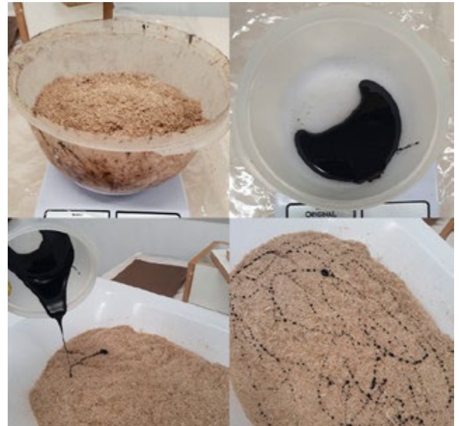
Figure 07: Preparation of the Fibers. Source: Authors.
