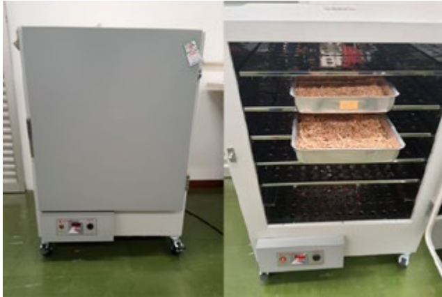
Figure 01: Drying and Sterilization Oven. Source: Authors.
