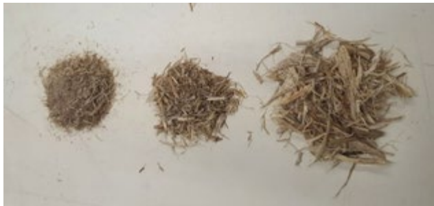
Figure 06: Sugarcane Bagasse Fibers Separated into Fine, Medium, and Coarse. Source: Authors.
