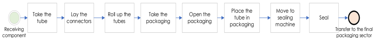
Figure 3 – Main production process for respirator extension hose
