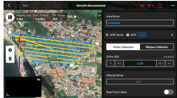
Figure 3. Flight plan with 2 cm GSD
