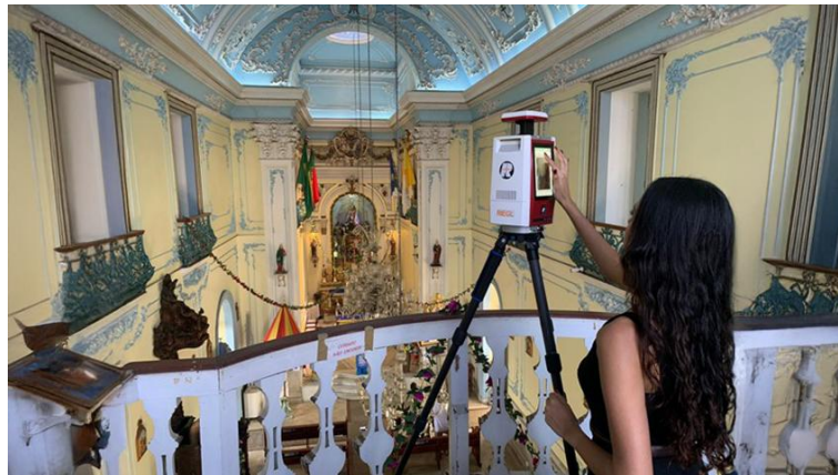
Figure 6. LiDAR surveying undertaken inside the church.
