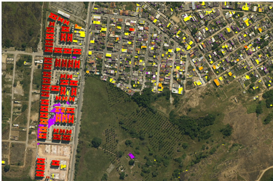
Figure 15. New construction in Santa Cruz. By crossing measured altitudes in the model, it is possible to determine if permits were properly followed.
