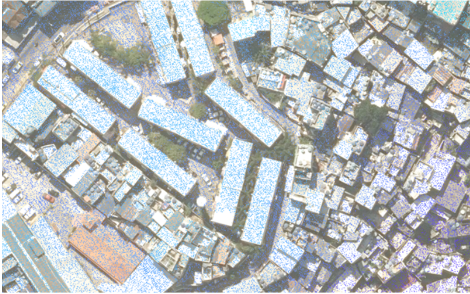
Figure 5. Filtered LiDAR point cloud showing classes 1 (ground), 2 (low vegetation), and 6 (building), over an orthomosaic. Both datasets are from the 2019 flight.
