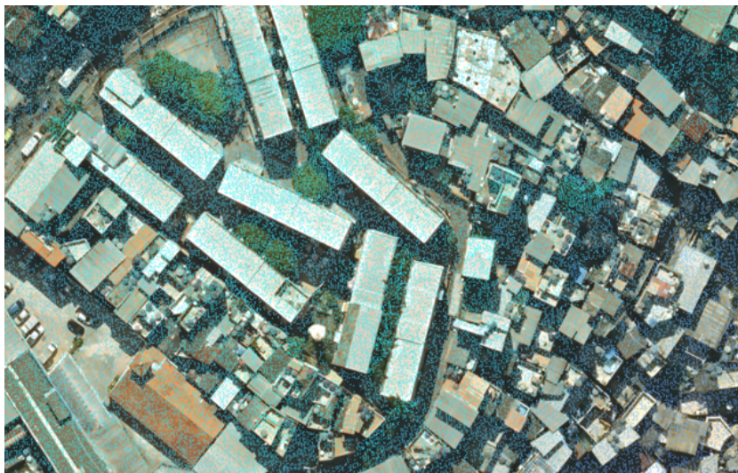
Figure 3. LiDAR point cloud (8 points/m 2 ) over an orthomosaic – both from the 2024 flight and covering an area of Rocinha, Rio de Janeiro
