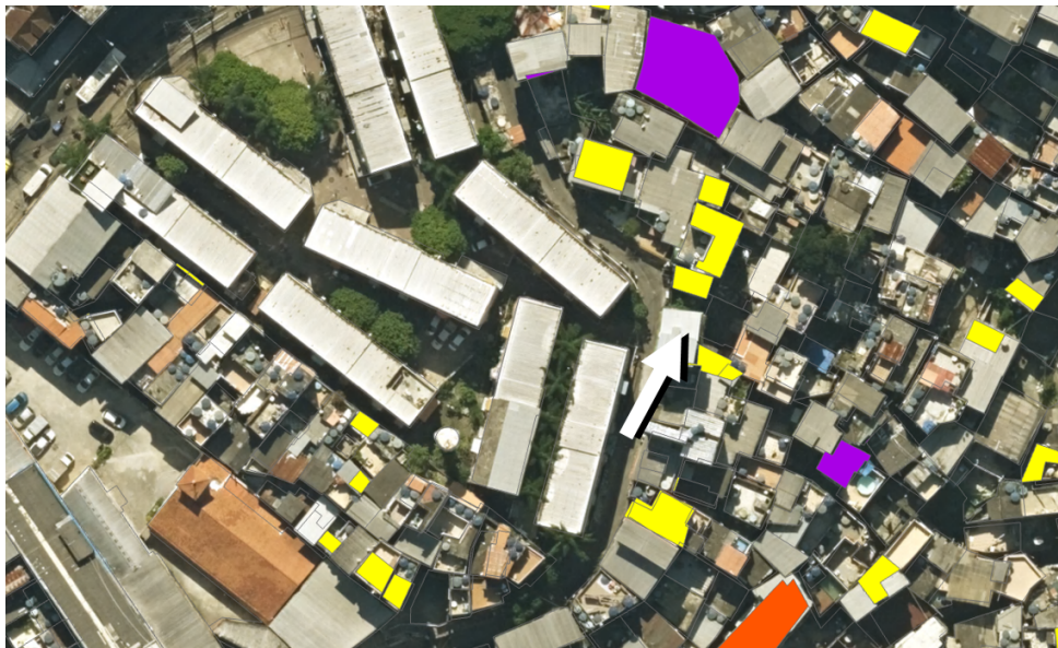
Figure 10. Zonal statistics (mean) per roof. Note that the building indicated by an arrow in this figure and in Figure 8 was not captured in the vector product because it did not exist in 2019.
