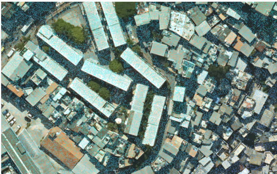
Figure 6. Filtered LiDAR point cloud showing classes 1 (ground), 2 (low vegetation), and 6 (building), over an orthomosaic. Both datasets are from the 2024 flight.
