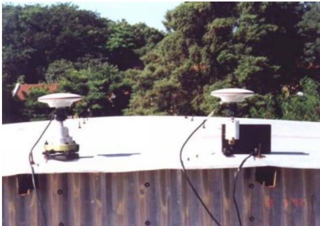
Figura 3 : Two GPS antennas over the aluminum roof and the rover antenna over the device
