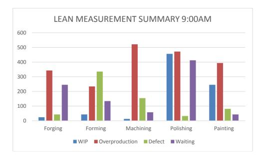
Figure 1 - Real-time data on the four types of waste of each workstation
